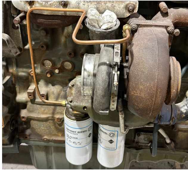
Turbo needs connecting elbows & new lube hose.
