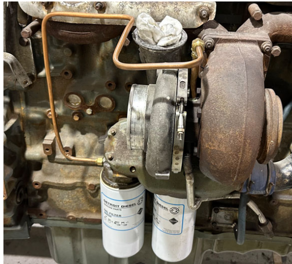
Turbo needs connecting elbows & new lube hose.
