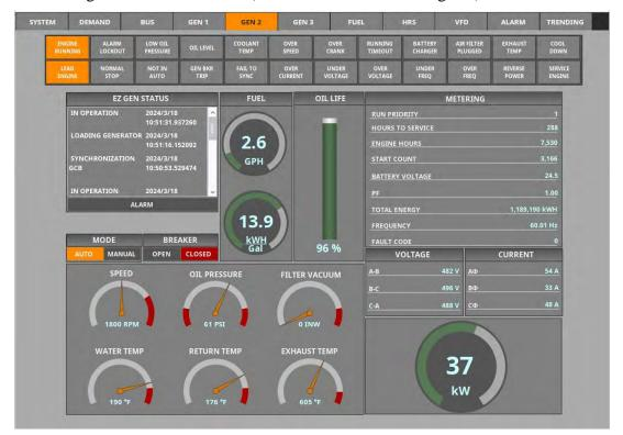
F. Engine-Generator Screen (for Gen #4 engine with charge air cooler):
