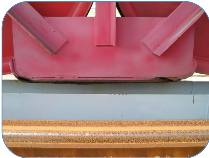
5.1.14 There was damage noted under the HV power cable directional reels.
