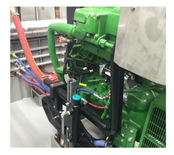
3. John Deere 6068AFM - Remove coolant tank and other accessories that are not required. Modify coolant discharge connection to face vertically at the front of the engine. Modify coolant suction connection to face horizontally at the front of the engine. See photographs below for representative installation.
