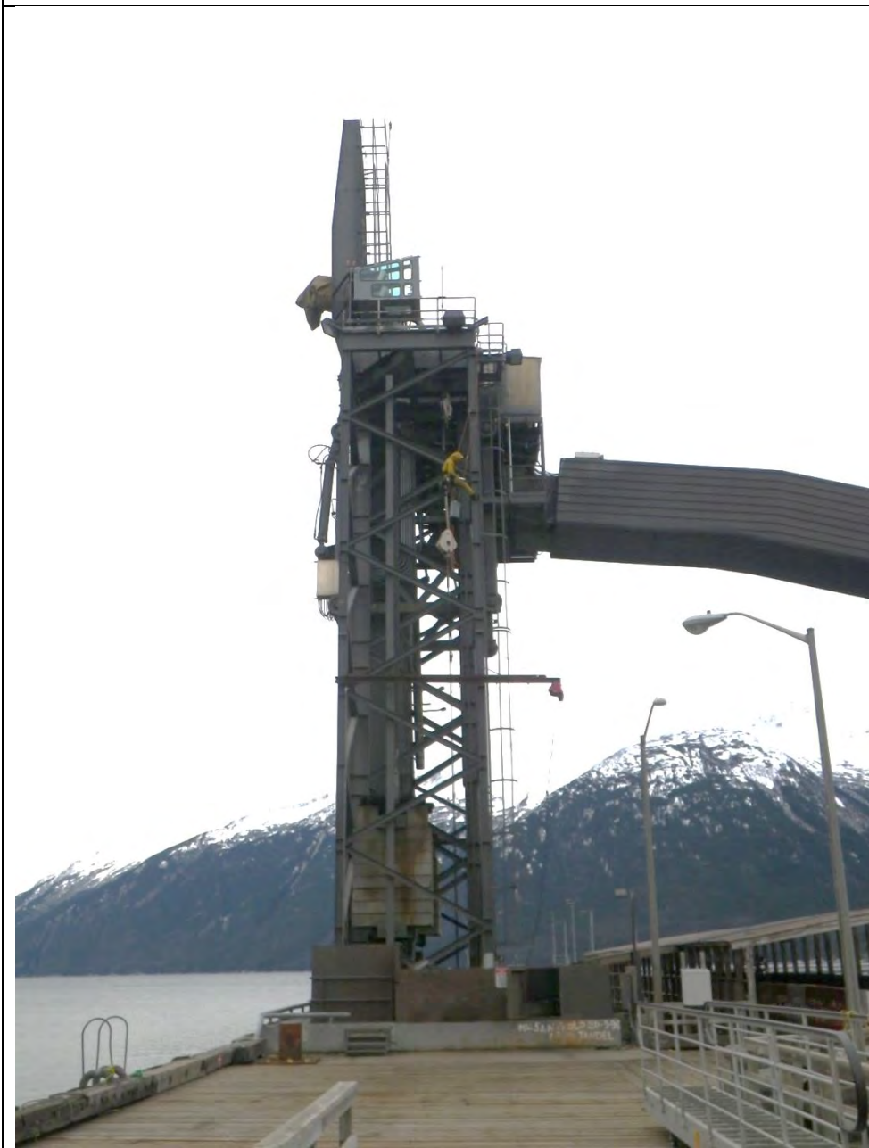
JKM-111213-IMG0285 LOCATION: SKAGWAY ORE TERMINAL SHIP LOADER DESCRIPTION: CLOSEUP VIEW (LOOKING SOUTH) OF NORTH SIDE OF SHIP LOADER WITH NO. 3 CONVEYOR ON BOOM IN PARKED POSITION (RAISED). INSPECTOR VISIBLE NEAR TOP OF TOWER.
