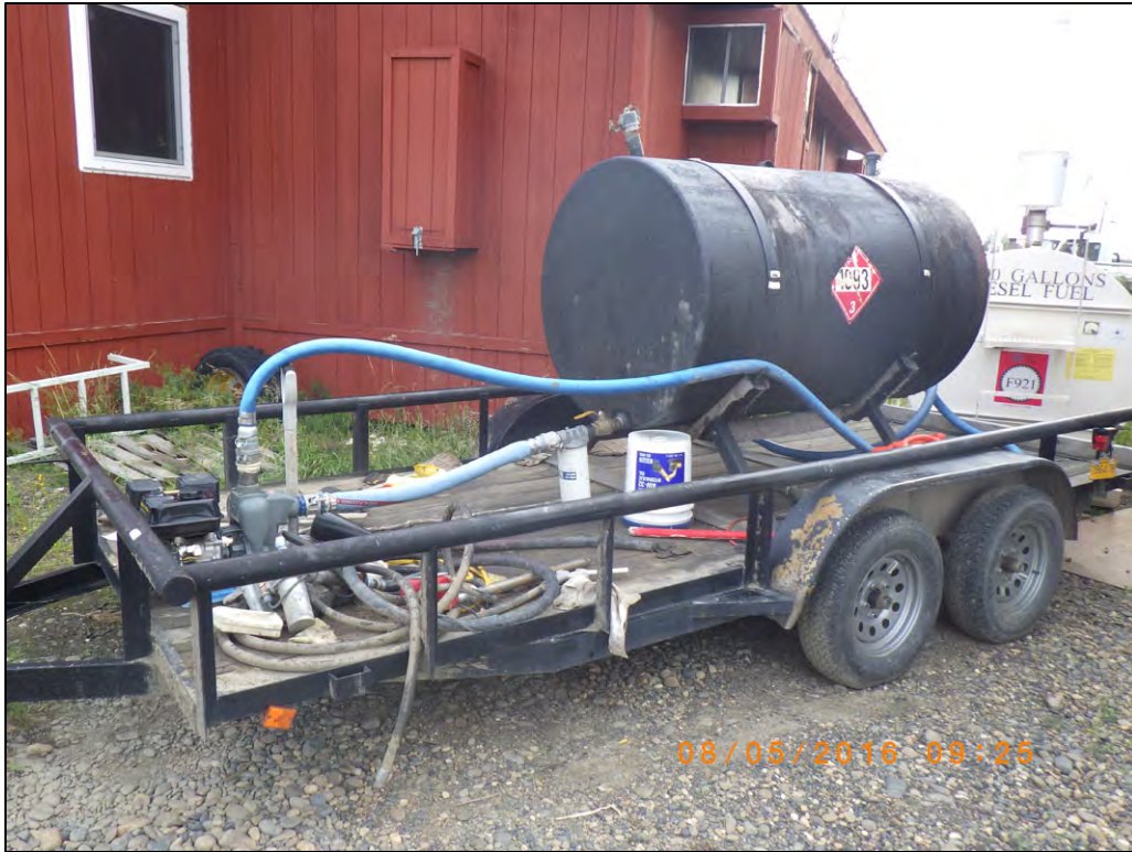
Photograph 13: 500 gal fuel trailer tank; generator house supply tank in background
