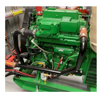
3. 6068AFM - Remove coolant tank and other accessories that are not required. Modify coolant discharge connection to face vertically at the front of the engine. Modify coolant suction connection to face horizontally at the front of the engine. See photograph below for representative installation.
