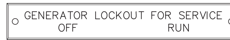
ENGINE CONTROL SWITCH – ECS
